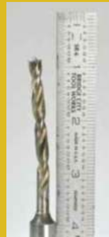
(Left) Bent drill bit
