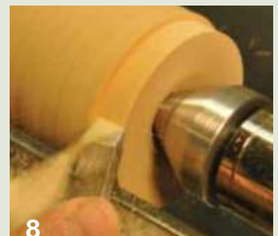
8 A peeling cut is useful for removing material quickly.
