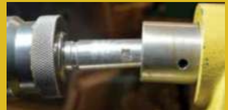
(Below) While drilling holes, a setscrew safely keeps the Morse taper of a Jacobs chuck in the quill of the tailstock.
