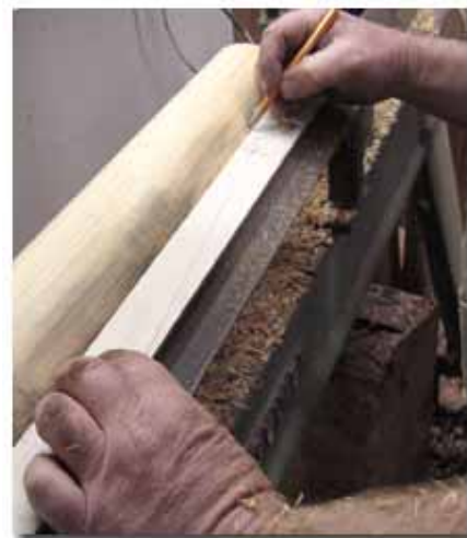
Using template to mark spindle
