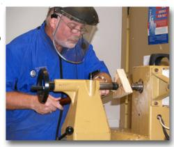
The initial turning is done between centers and Joel uses a stebcenter (made by Robert Sorby) in the spindle to drive the blank and to turn a tenon for the scroll chuck. A two or four
