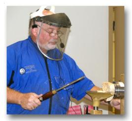
The blank is then installed in the scroll chuck to complete the turning.
