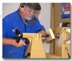
The initial turning is done between centers and Joel uses a stebcenter (made by Robert Sorby) in the spindle to drive the blank and to turn a tenon for the scroll chuck.
