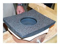
Here he shows an example of a wide rimmed vessel. He uses a home made vacuum vice to hold it in place while it is being turned.
