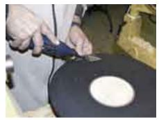
A power chisel type of carving tool is then used to cut the pattern after drawing a pattern on the rim. --->
