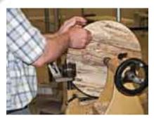
Larry Walrath began his program on using the McNaughton Center Saver by rough turning a large spalted blank and then mounting it on a large faceplate. A scroll chuck does not have enough grip to keep from slipping and breaking loose when using the McNaughton Center Saver. The blank is then mounted on the lathe and the Center Saver is used
