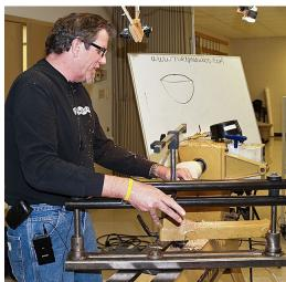
After the exterior is finished, the hollowing process begins. After the initial hollowing, Steve used a captive bar hollowing rig to complete the hollowing process.
